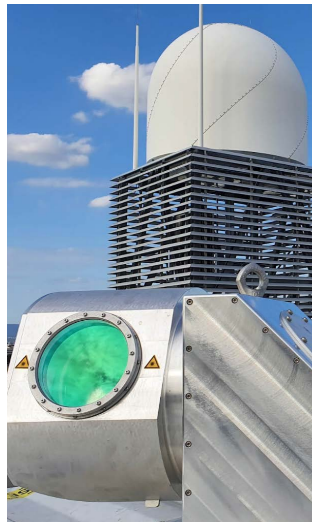
SKIRON3D lidar in combination with a Leonardo X-Band weather radar
